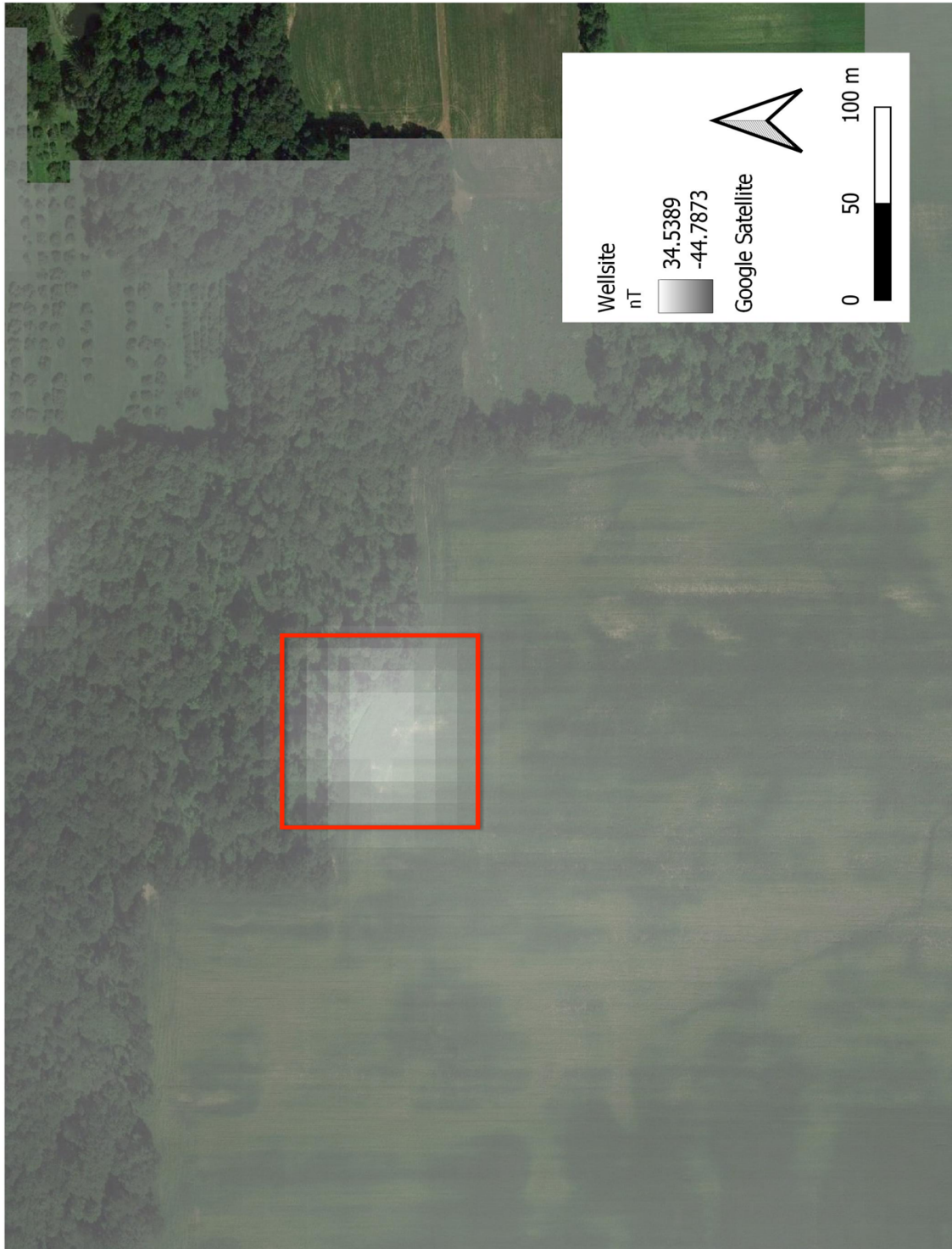
FIGURE A3 – Wellsite 375991001: Identified area of interest identified for terrestrial survey as part of the proposed follow-up survey effort. Grey overlay indicates results of previously collected aeromagnetic dataset with white color indicating peak positive magnetic intensity values.
